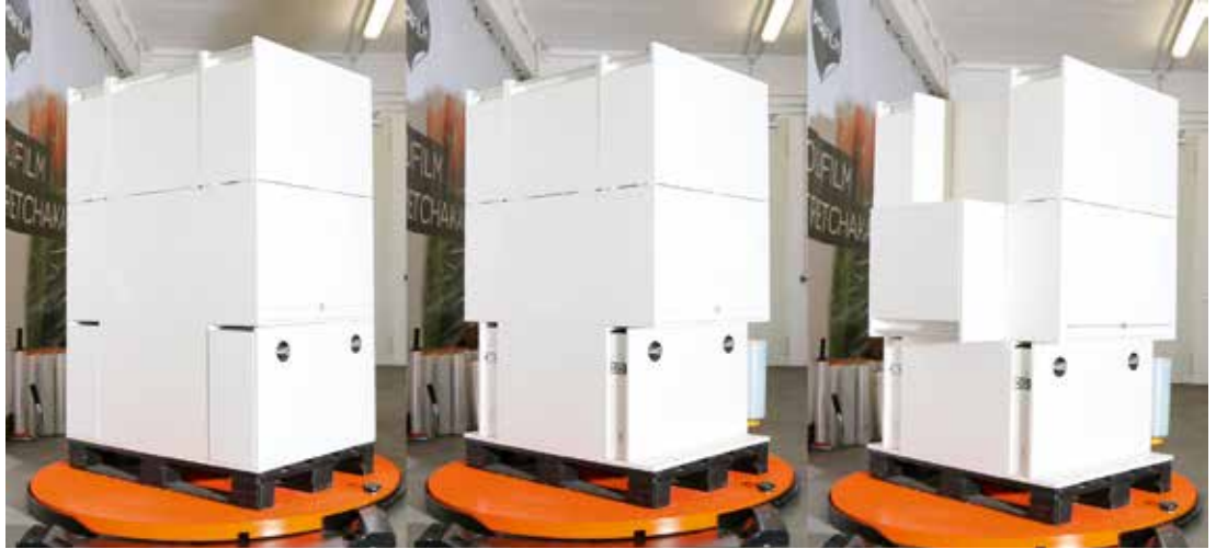
Fig. 1. Different-shaped load units: straight and flush with the pallet (left: type A), with protrusions above and/or below (middle: type B) and very unevenly arranged goods (right: type C)
