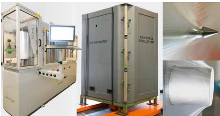
Fig. 5. Test equipment and process: FPT-750 from ESTL (left) and practical test on the test pallet (center) with puncture and plate test (right) (© Polifilm)
